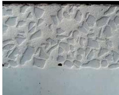
Laser cladding creates an atomic bond between substrate and top layer. Metallurgical they become one. This makes the cladding layer super strong.
